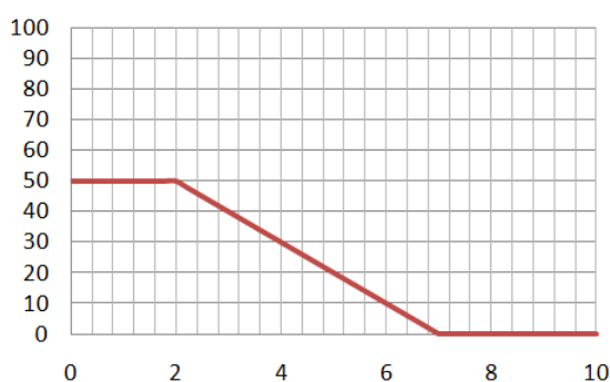
FIGURE 7. Secondary Air dependence on oxygen concentration
