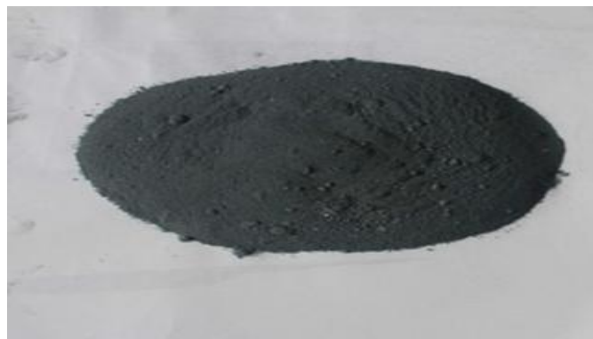
Fig 2: Condensed Silica Fume (CSF)
