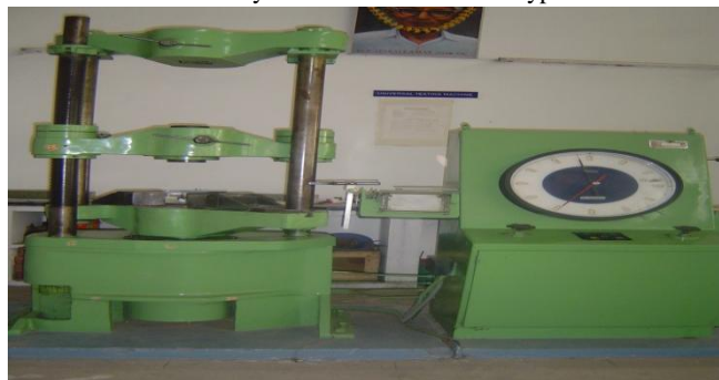
Fig 11: universal testing machine with three point loading arrangement used for the flexure test
