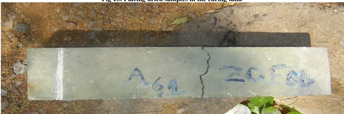
Fig 19: Failure pattern in concrete beams after flexure test was carried out on them
