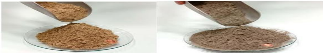
Fig1: Class C (left) and Class F (right) Fly Ash
