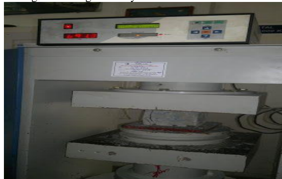
Fig 9: Compressive testing machine that was used to test the strength of the cubes
