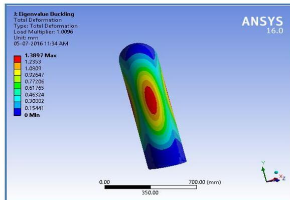
Figure 13 First Buckling for 160 gsm
