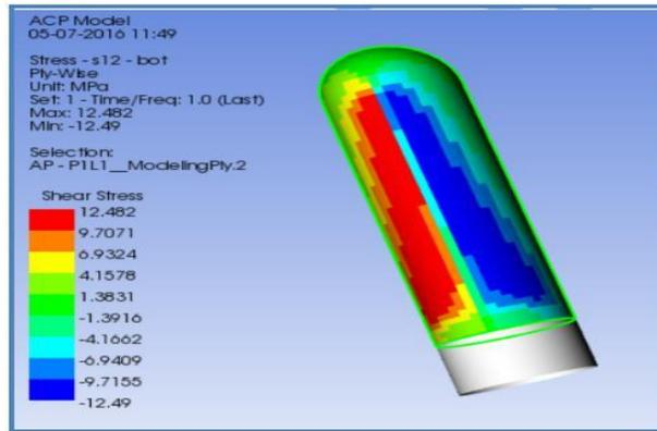
Figure 10 In plain inter lamina Shear Stress (220gsm)
