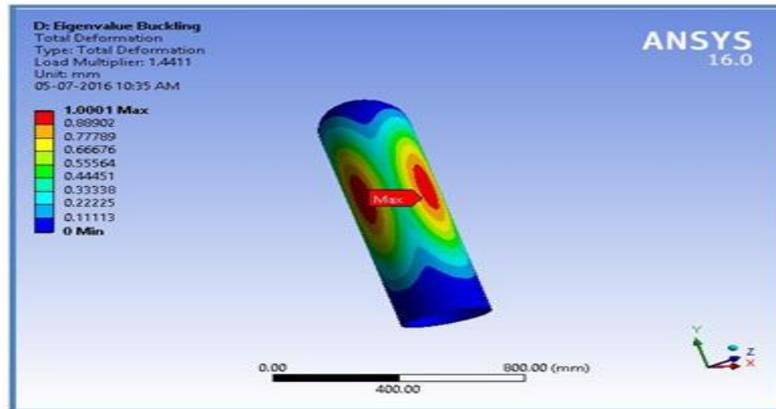
**Figure 14** First Buckling for 220 gsm
