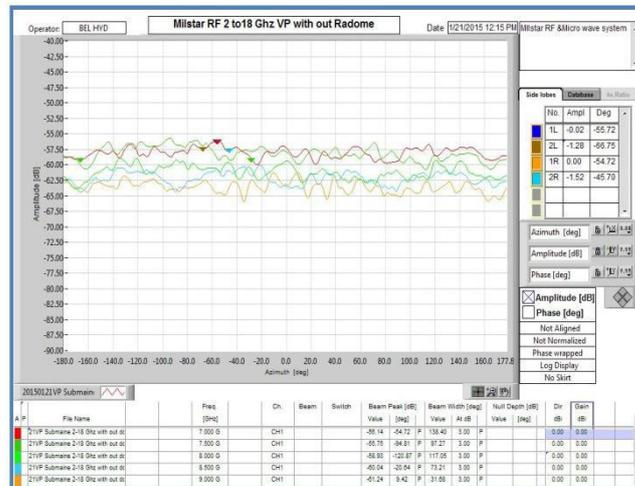
Figure 1 Insertion loss properties – Vertical polarization
