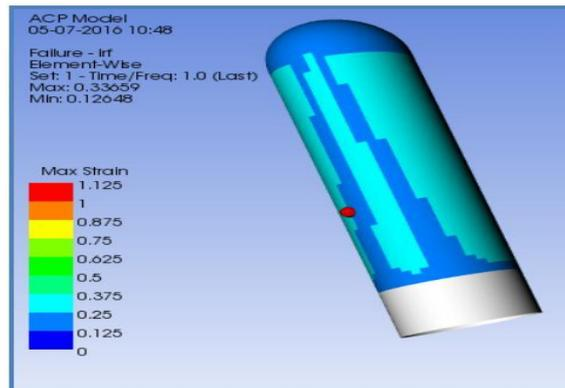
Figure 12 Max strain for 220 gsm
