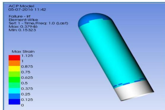
Figure 11 Max strain for 160 gsm
