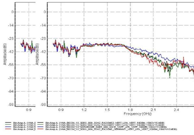
**Figure 18** Insertion Loss of radome at various heights
