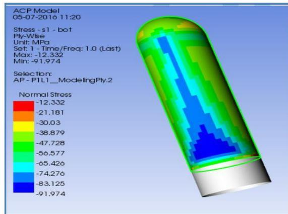
Figure 7 Normal stress (160 gsm)
