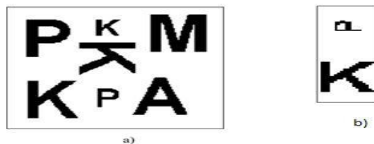
Fig .1 illustrate a pattern recognition based on the template matching approach. Fig .1.a is the input image I, Fig.1.b represents two templates (K representing letter 'K' and P letter 'P').
