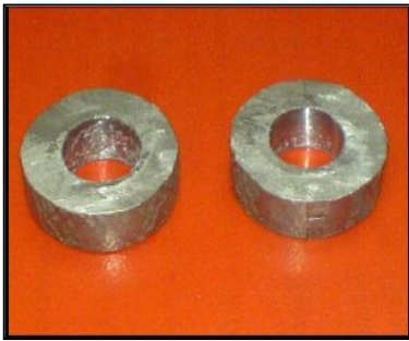
Fig 2.2. rings before compression
