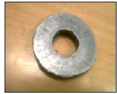
Fig 2.3. rings after compression
