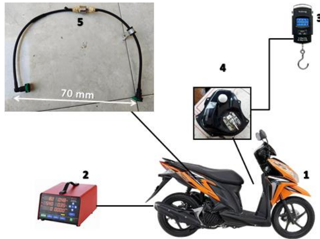
Figure 1. Testing equipment schematic. 1. Motorbike, 2. Exhaust gas analyzer, 3. Digital spring scale, 4. Fuel tank, 5. Fuel line
