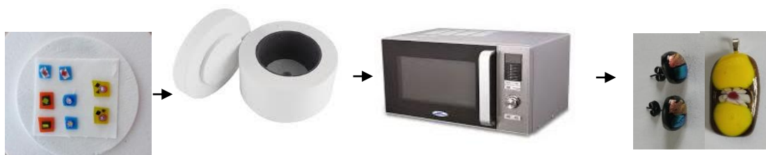
Figure 1. Schematics of microwave glass formed jewellery process
