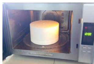
Figure 4: Layered glass ready for microwave fusion
