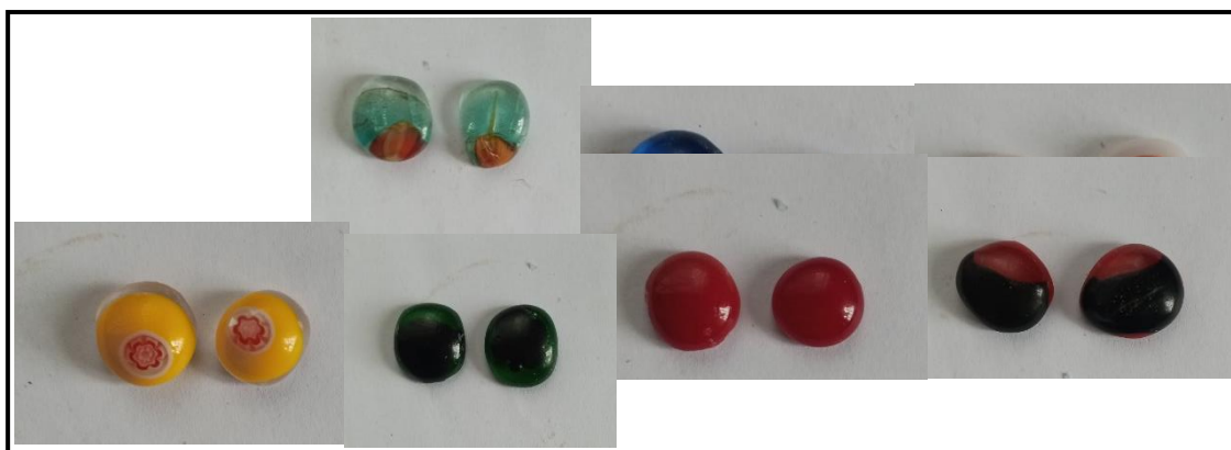
Figure 6. fully fused glass forms.
