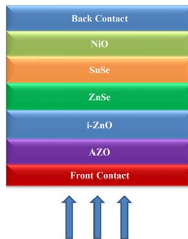
Figure 5.1: Arrangement Of 5 Layer Thin film Solar Cell.
