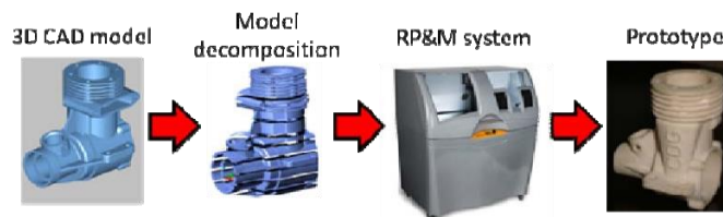
Fig. 1. RP&M general procedure to construct a component.
