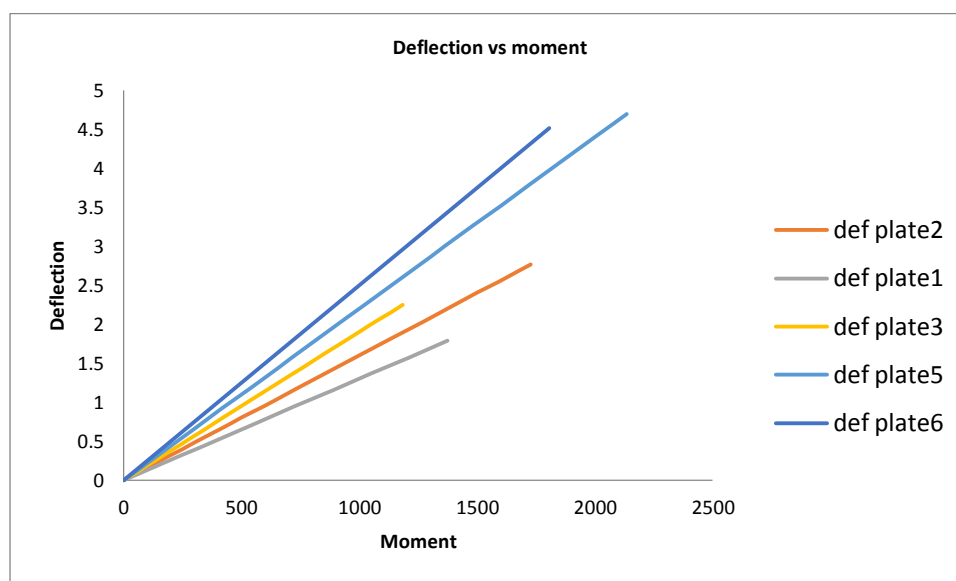
Fig 4.6: Experimental Deflection (mm) vs Moment (KNm) for all plates
