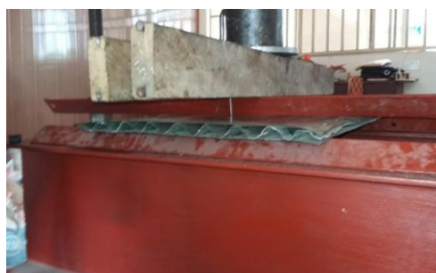
Plate 2: Sandwich plates with sinusoidal corrugated core
