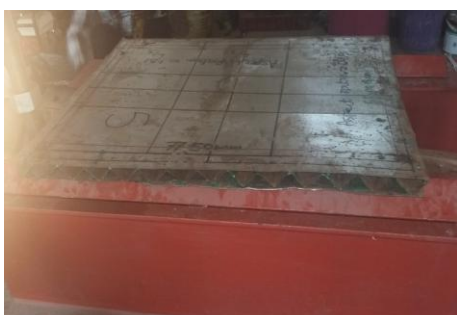
Plate 3: Sandwich plates with triangular corrugated core
