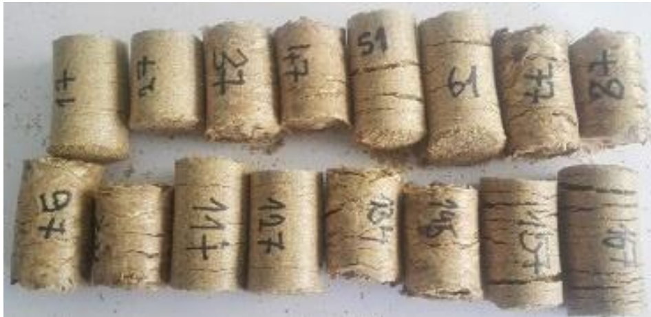
Figure2. Samples – briquettes from acacia wood produced during the experiment
